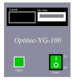
5. To activate the mercury lamp, hold the "trigger" switch for a second or two. The current should go up to around 9.50 Amps. It will then drop down to around 4.80 Amps as the lamp comes on. There are multiple laser settings for multiple colors. You can use the laser color setting toggle to select blue or green. The blue setting engages a yellow filter to filter out blue light. The green setting has a red filter to filter out green light.
