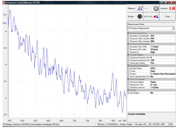
5. To save the spectrum, first, close the measurement result, and a new window with the previous data will be displayed. Save the data from "File – Save as".
