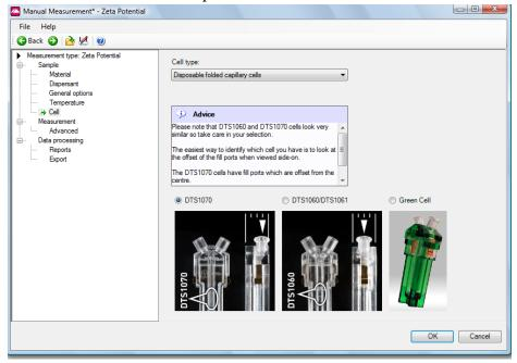
5. Once saved the manual setup, you can recall it in the future to repeat measurements, or make any edits based on the saved setup parameters. A window of the measurement will appear after setup. Mount your sample cell in the holder and start measurement.
