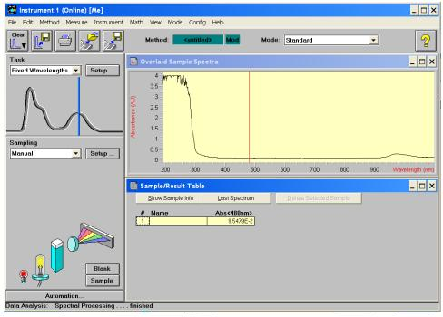
6. The transmittance spectrum can be calculated by going to "Math" – "Transmittance". Save the data from "file" – "export the selected spectrum".
