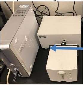
3. Run the software "Instrument 1(online)" on the desktop. Wait for the connection between the spectrophotometer and the computer. Click on the lamp and select "Lamp ON". This will turn on the lamp for an excitation light source.
