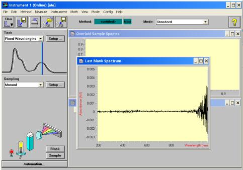
5. Next, load the sample solution in the same type of cuvette and click "Sample". The absorbance spectrum is measured and displayed.
