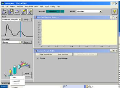
4. Load an empty cuvette and click "Blank". A blank spectrum will be measured and displayed.
